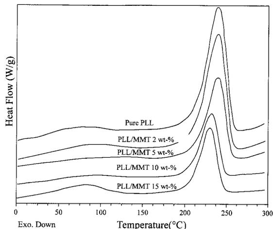
**Figure 4.** Comparison of DSC thermographs for all relative PLL to MMT compositions studied (graphs are offset vertically for clarity).
