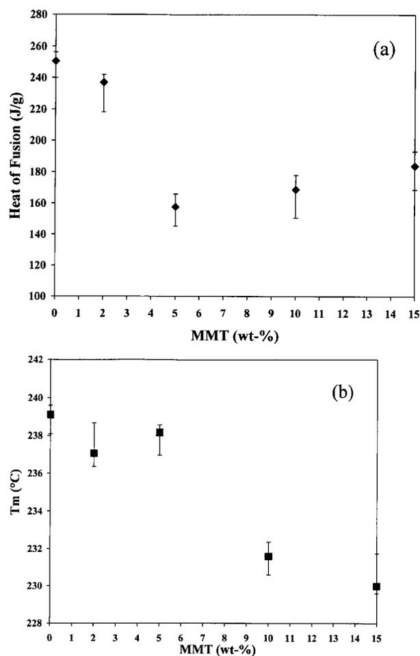
**Figure 5.** (a) Heat of fusion and (b) melting point variations of PLL/MMT nanocomposites with respect to clay composition. In both (a) and (b), the results of three measurements are exhibited by the data point representing the middle observed value, and the error bars represent the total spread of the three measurements.
