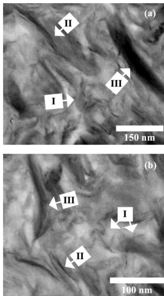
**Figure 3.** (a) and (b) TEM bright field images of semi-crystalline PLL/MMT (10 wt % MMT) nanocomposite showing a mixture of intercalated clay tactoids (I), exfoliated clay platelets (II), and clay platelets parallel to the material cross section/normal to the electron beam (III).
