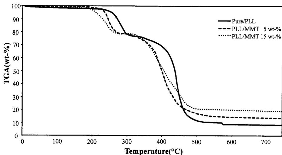
**Figure 6.** PLL weight loss from TGA scans for 5 and 15 wt % MMT in PLL nanocomposites and pure PLL.
