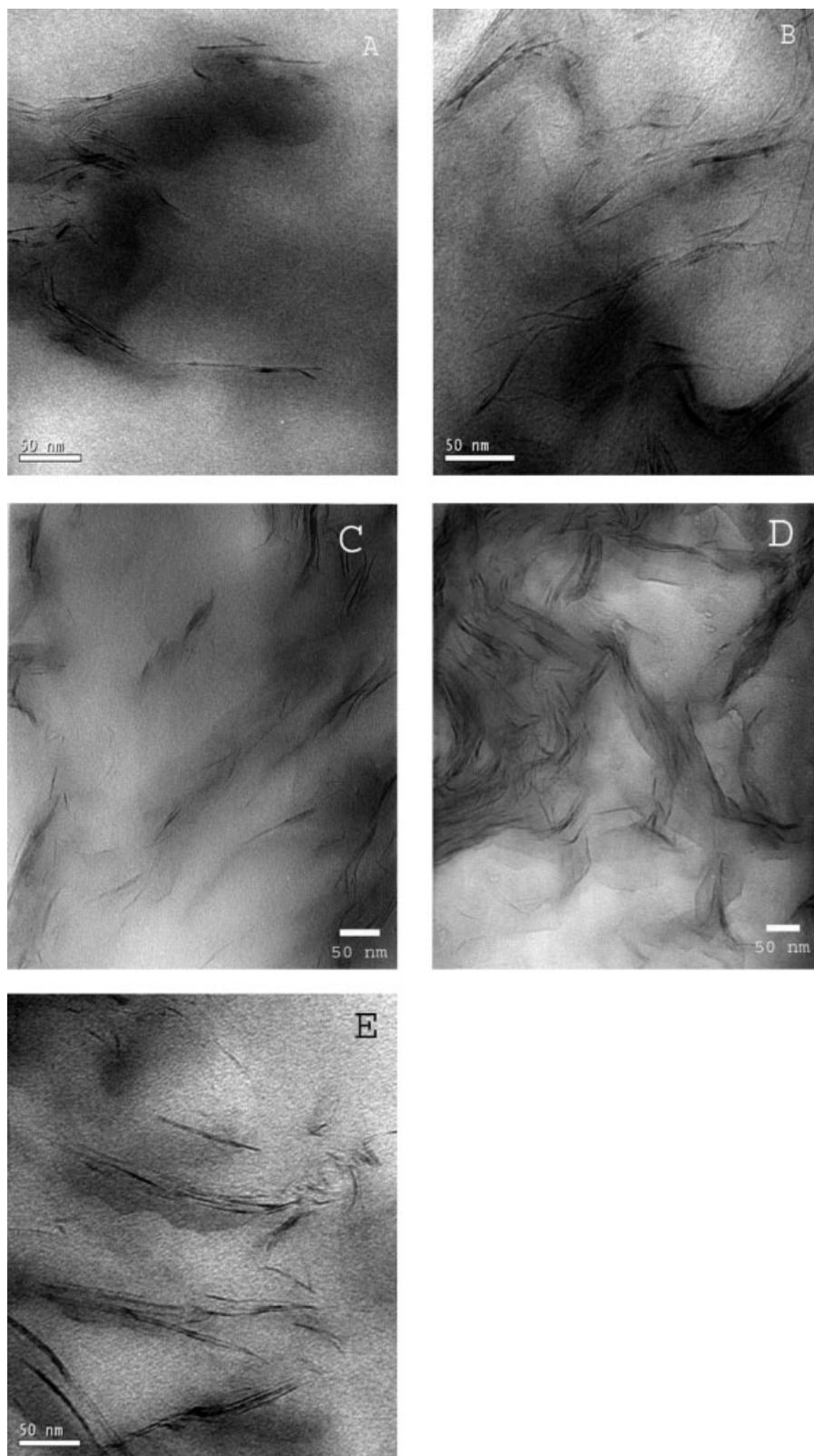
**Figure 8.** Bright field TEM images of 2 wt % (A), 5 wt % (B), 10 wt % (C), 15 wt % (D), and 2 wt % in low molecular weight (25,500 g/mol) (E) PLL-MMT nanocomposites, showing intercalated regions. Images were obtained on microtomed films (<80 nm) at 200 kV.
